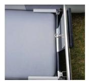
Insert D-Rings on the bottom of the air deck floor, through the slots in the boat floor fabric layer. Lash the two D-Rings together with the included webbing strap.
