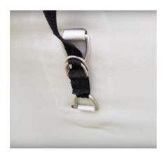
8. Inflate the floor to 10 psi. While inflating the airdeck floor, be sure to pause and walk on the floor to push it into place. Don't forget to activate the check valve by pressing down on the centre pin and turning it ¼ turn in either direction. If it is popped up it wont let any air escape. When taking the pump out, do it quickly as you wont loose much air.
