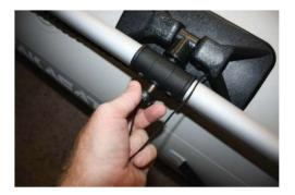
11. If you opted for the Quick Release Wheels, install them now in the down position. When in the down position, the wheels provide enough heigh to mount a 15" short shaft outboard in the upright position.
