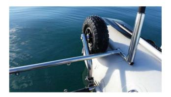
13. After launching your boat into the water, check the pressure in the hulls to verify you still have 3 psi hull air pressure. If the water is cooler than the air temperature, the air inside the hulls will condense causing a pressure drop. Use the manual pump to inflate back to 3 psi hull pressure if needed.
