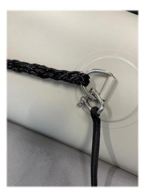
3. The Ring can be fitted between the D-Rings Underneath the Deck for towing or Float between the D-Rings on the tube and the Floor D-Rings for Anchoring or a higher tow point.
