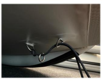
2. Connect the D-Shackles to the Inboard D-Rings on the Bow of each tube.
