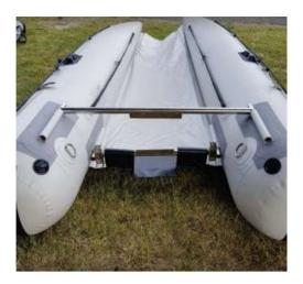
5. Slot the smaller motor mount board inside the Tube Transom.
