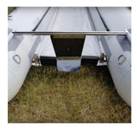
6. Creating a sandwich, assemble the rest of the transom. The bolt passes from the rear to the front with the rubber washer between the wooden motor mount boards.
