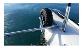
14. After launching your boat into the water, check the pressure in the hulls to verify you still have 3 psi hull air pressure. If the water is cooler than the air temperature, the air inside the hulls will condense causing a pressure drop. Use the manual pump to inflate back to 3 psi hull pressure if needed.
