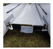
4. From the front, insert the upper transom bar into the upper set of tubes on the boat hulls. The stainless tab should be facing down when insert properly.
