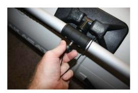
12. If you opted for the Quick Release Wheels, install them now in the down position. When in the down position, the wheels provide enough heigh to mount a 15" short shaft outboard in the upright position.
