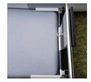
8. Insert D-Rings on the bottom of the air deck floor, through the slots in the boat floor fabric layer. Lash the two D-Rings together with the included webbing strap.
